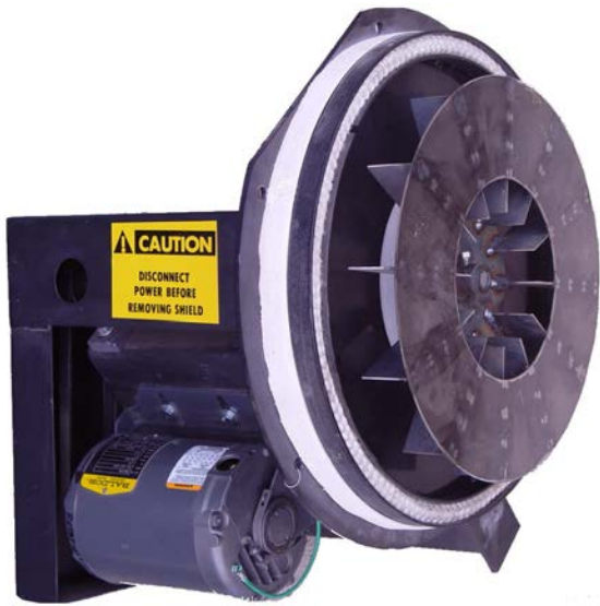
Figure 28: Belt-drive fan assembly removed from boiler and showing white gasket
